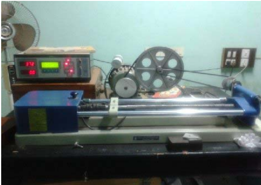
Figure 2 Digital tensometer setup (see online version for colours)
